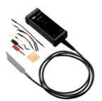
The ZS Series probes provide high impedance and an extensive set of probe tips and ground accessories to handle a wide range of probing scenarios. The high 1  $\mbox{M}\Omega$  input resistance and low 0.9 pF input capacitance mean this probe is ideal for all frequencies. The ZS Series probes provide full system bandwidth for all Teledyne LeCroy oscilloscopes having bandwidths of 1 GHz and lower.
